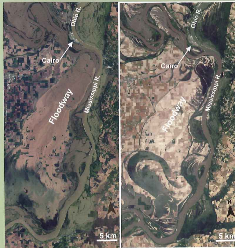
Birds Point-New Madrid Floodway (left) after levee breach (May 3, 2011) and (right) after Floodwaters receded (June 4, 2011). Images From NASA Earth Observatory.
